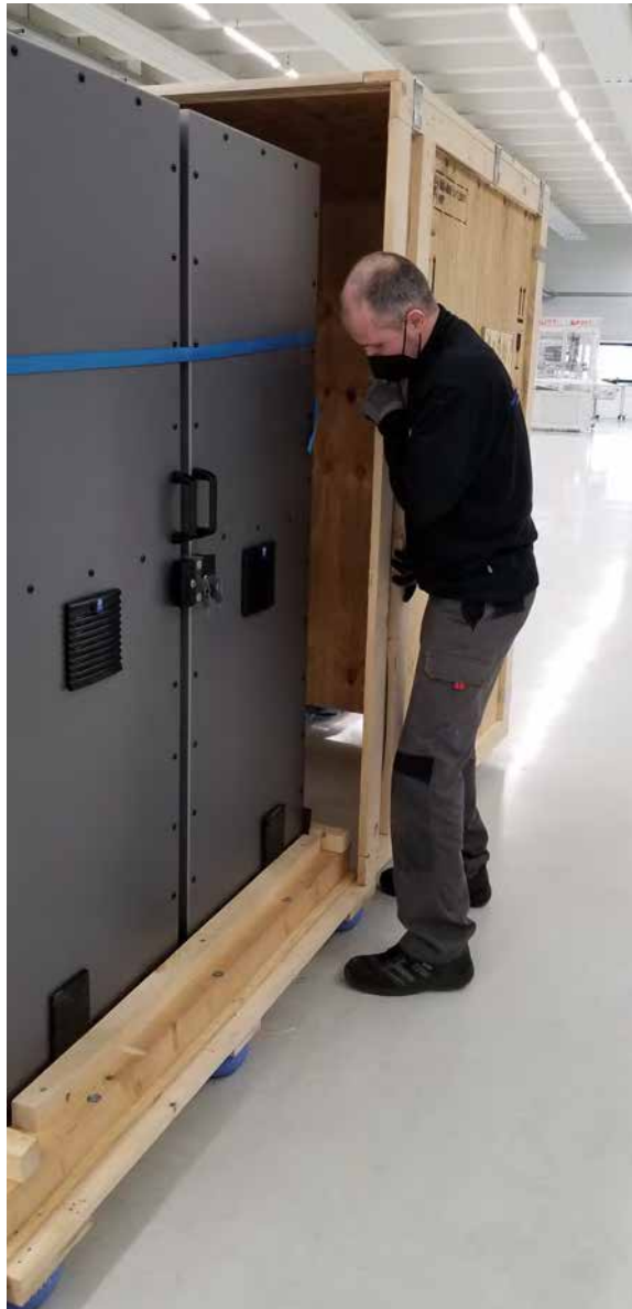
Figure 7 Remove crate body from the pallet (Rack packing material not shown)
