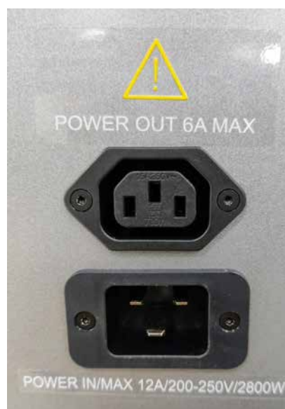
Figure 14 Power Input and Power Output Connectors
