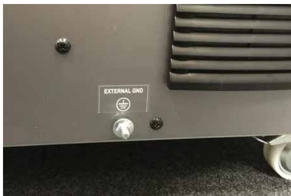
Figure 12 External Ground Connector on right side of Rack
