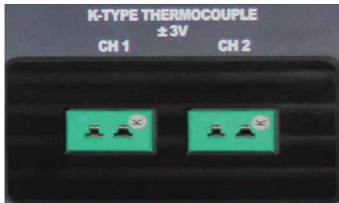
Figure 37 Type K Thermocouple Jacks on Test Fixture Front
