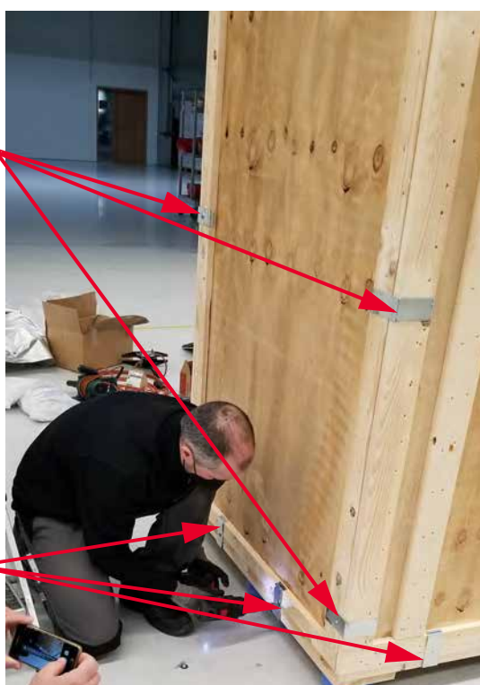
Figure 6 Remove clamps securing crate to pallet
