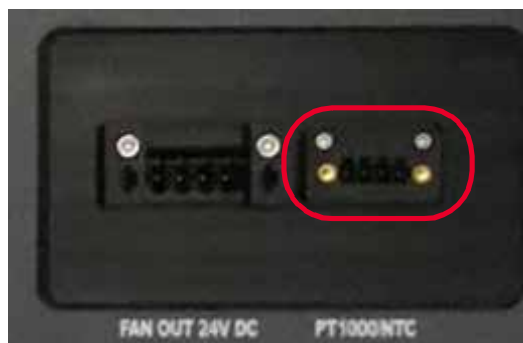
Figure 35 NTC Connector on Front of Test Fixture
