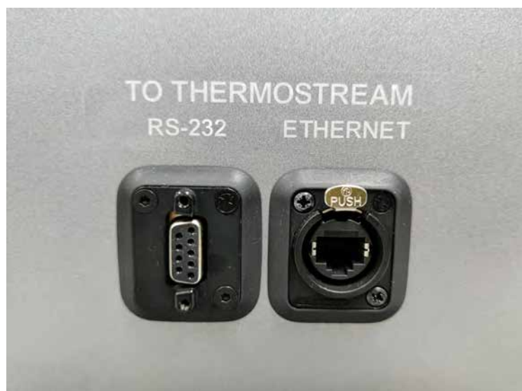
Figure 43 Thermostream RS-232 and LAN Connection on PD1550A Rack
