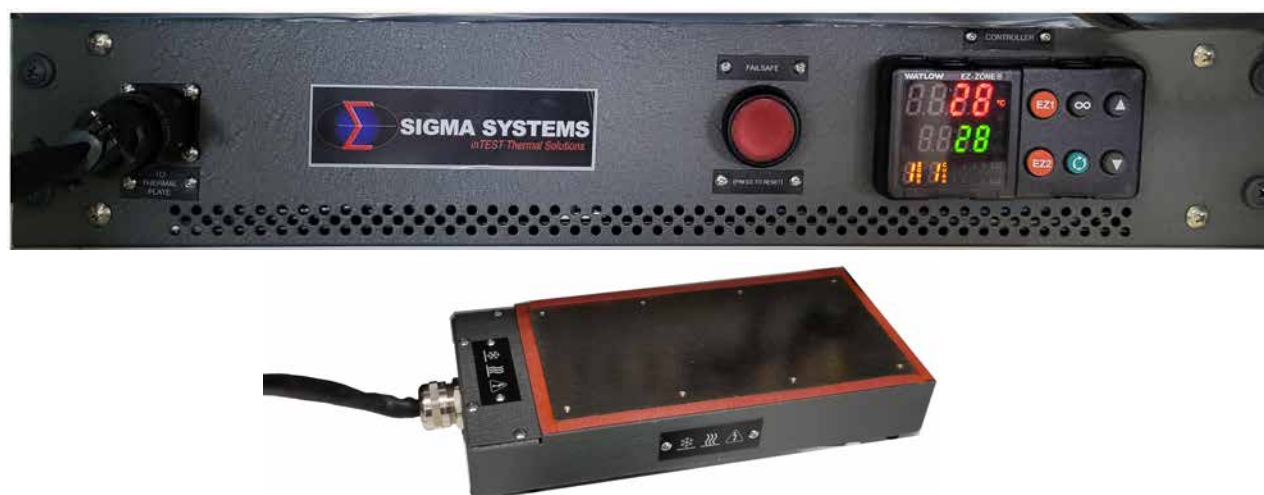
Figure 38 InTEST (Watlow) Controller Unit in Rack Panel and Heating Plate
