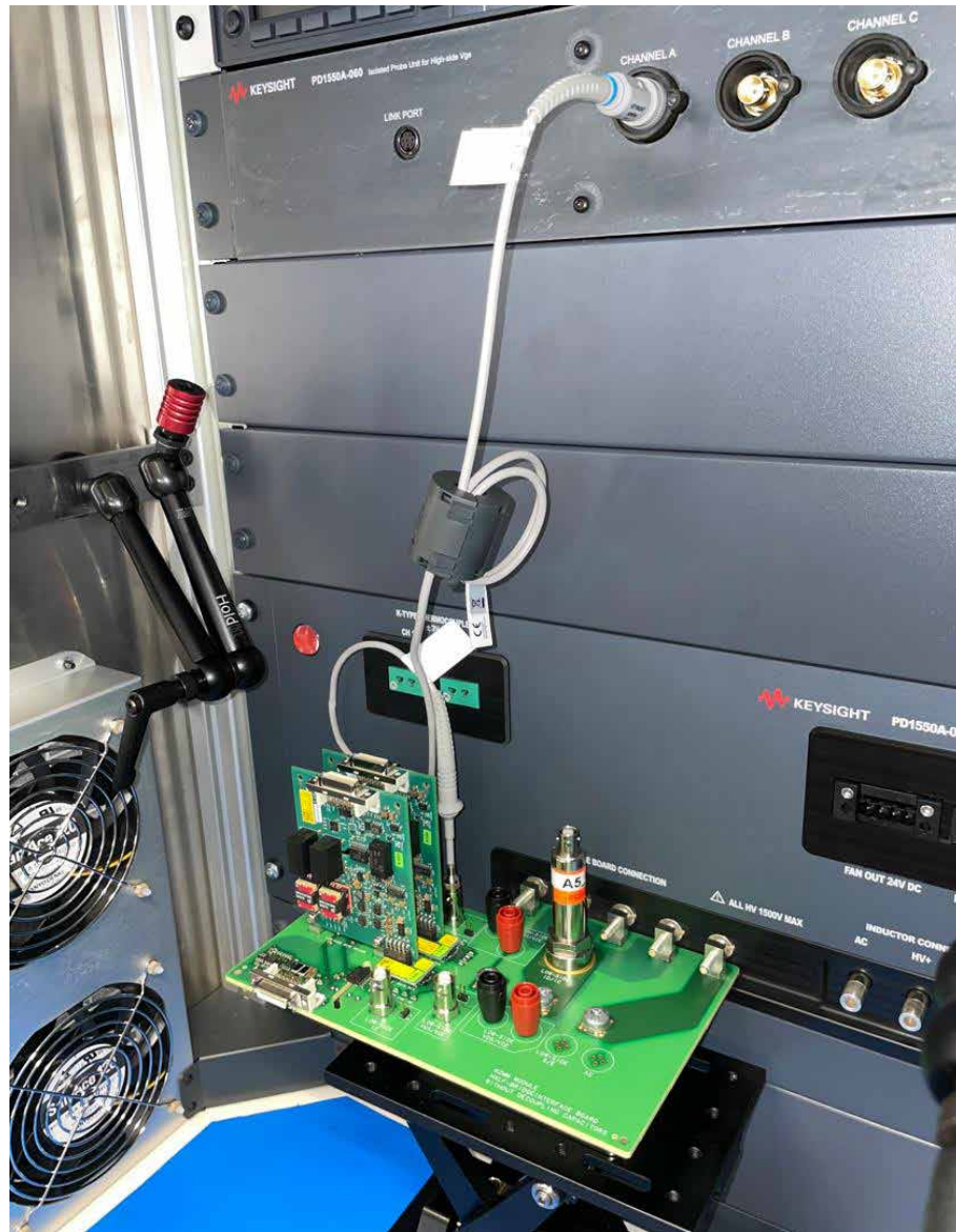
Figure 31 N2873A Probe to High-Side Gate Voltage V_{GS,H}/V_{CE,H} and Channel A on Isolated Probe Unit
