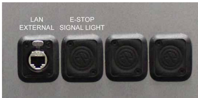
Figure 13 External LAN and Emergency Stop Connectors
