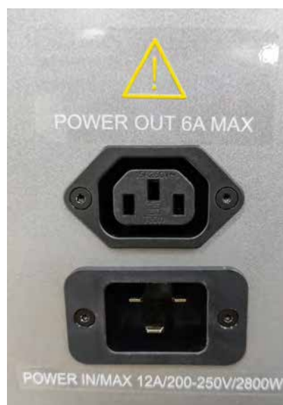
Figure 14 Power Input and Power Output Connectors
