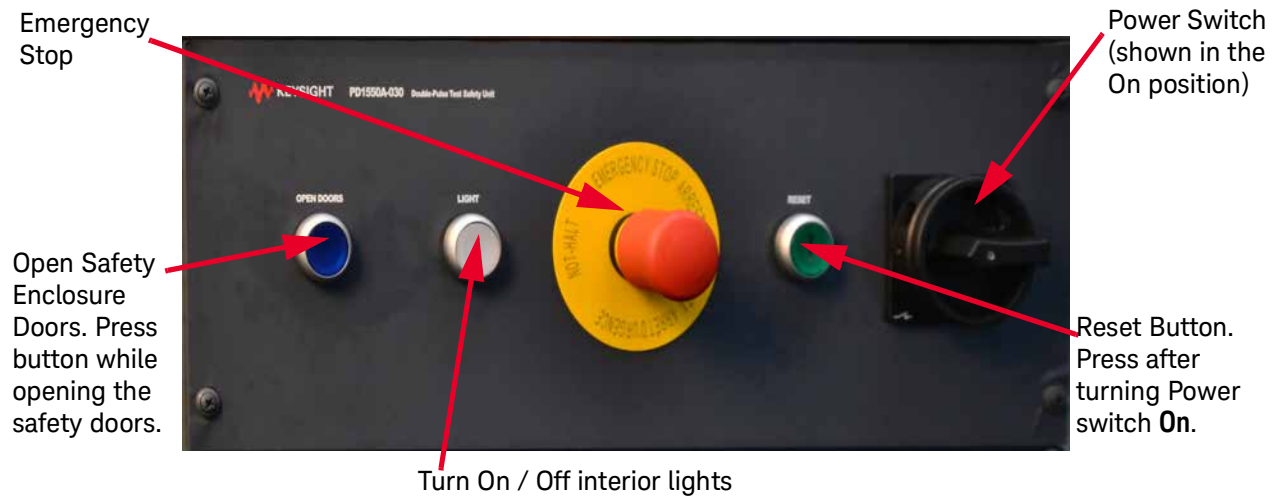
Figure 2 PD1550A-030 Safety Unit (Power switch shown in the On position)
