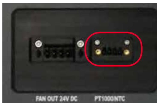
Figure 35 NTC Connector on Front of Test Fixture
