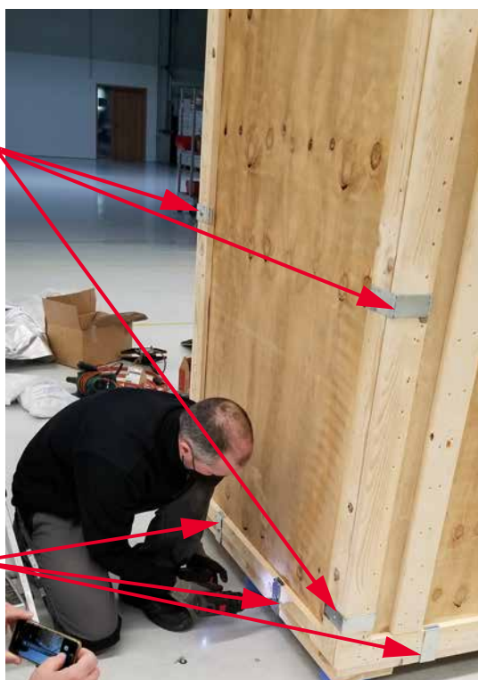
Figure 6 Remove clamps securing crate to pallet
